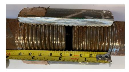
Slide 15 of Mr Southward's presentation which shows two rebar with 44mm threads, with one fully engaged and two threads exposed on the other
