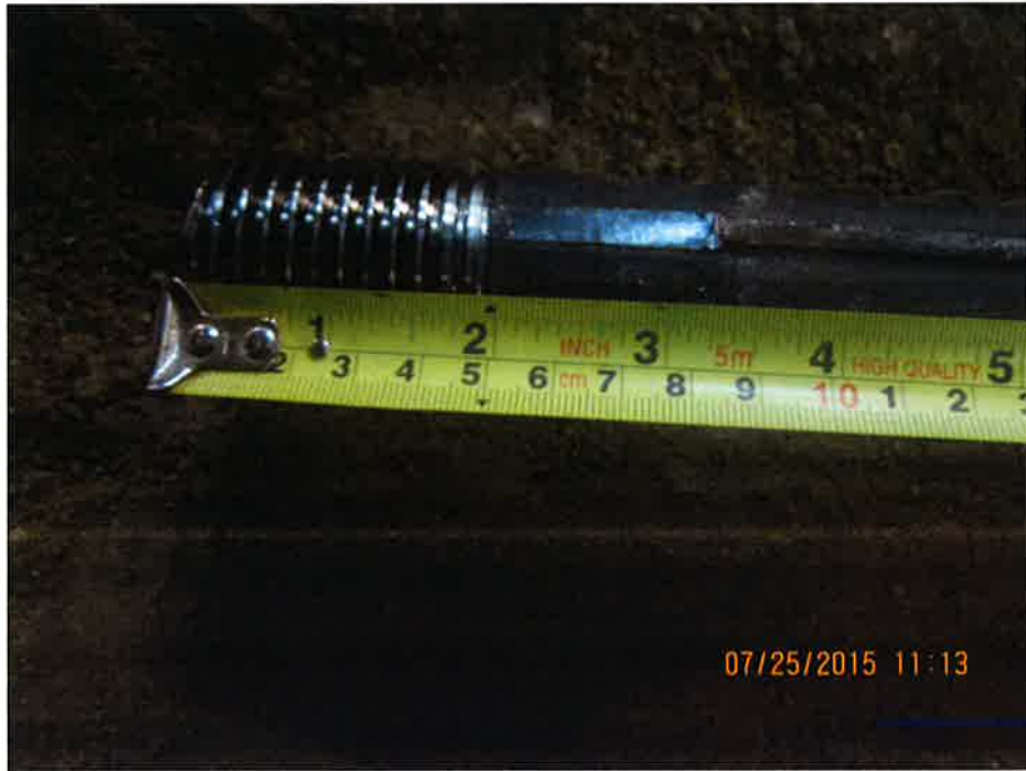
Image 4 – random checking of Type A threaded rebar (Y40) for 3m EWL slab in Area C1-1.
